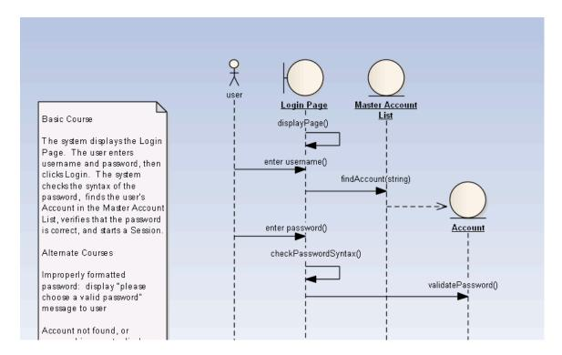
Once the Sequence diagram is completed, the Add-in is used to generate unit tests from the messages on the Sequence Diagram. Note that "controllers" on Robustness diagrams tend to reflect a slightly higher abstraction level than Sequence messages; that is, a controller may be implemented as multiple messages on a Sequence diagram.
