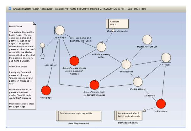
By analyzing our use case using the Robustness Analysis technique, we've added a lot of information to the model that can be used to drive the testing of the application. To begin with, our add-in can automatically generate test cases for each "controller" on the Robustness diagram.
