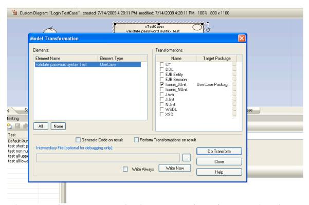
When we transform our test case using the ICONIX JUnit transform, "setup()" and "tearDown()" methods are added automatically, and a test method is created for each scenario. This transformation, originally envisioned by Matt Stephens while we were writing the book "Agile Development with ICONIX Process<sup>1</sup>", and implemented by Sparx Systems, is the essence of the Design-Driven Testing approach.
