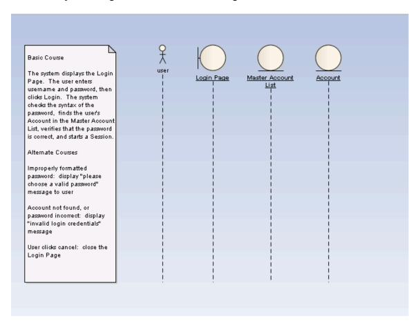
The add-in automatically creates a new sequence diagram, and brings a "hot-linked" note, and all Boundary and Entity objects from the Robustness diagram onto the Sequence diagram. Developers then complete the design of the use case on the Sequence diagram.
